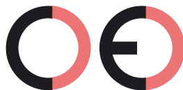
False CE Mark (too far)
